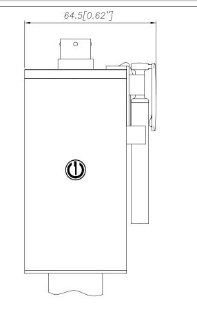
The Autozero function is activated through a magnetic contact (external magnet supplied with the sensor).
